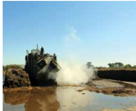
Ruben Lopez operates the "cross mix turner" at the mushroom farm. It straddles the compost rows and turns them upside down as it mixes the compost. Photo by Barbie Lange
